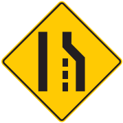
Right lane ends ahead
