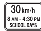
School zone. The tab underneath indicates the speed limit and the hours that it is in effect (in this case, the 30 km/h limit is in effect from 8 a.m. to 4:30 p.m. on school days)
