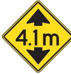
Low structure clearance 4.1 metres
