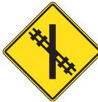
Railway crossing advance warning, track position indicates the angle the railway tracks cross the road
