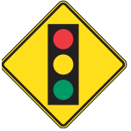
Traffic signals ahead
