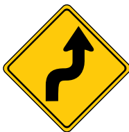
Reverse curve ahead Two turns in opposite directions separated by a tangent of less than 120 m, first turn right
