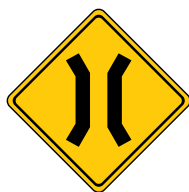
Narrow bridge ahead Width of pavement narrower than approach
