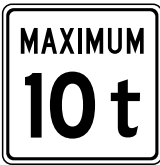
Weight limit of vehicle permitted on highway or bridge expressed in tonnes
