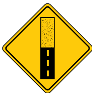
Pavement ends Continuation has gravel surface
