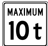
Weight limit of vehicle permitted on highway or bridge expressed in tonnes
