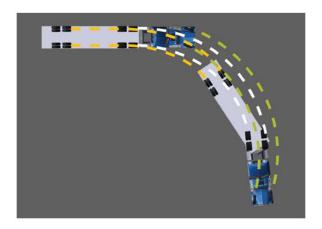
The combination unit of a truck-tractor and "pup" trailer has different turning characteristics than those of the semi trailer type. These units have turning radius and off-track patterns within each unit, but the amount of off-track is dependent upon the length of the draw bar and the wheel base of the units.
