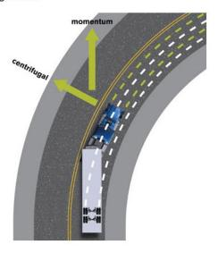
The degree of control you are able to maintain over your vehicle is determined by the amount of traction your vehicle's tires have with the road surface. Entering a curve too fast can result in skidding or a rollover. Applying brakes in a curve can cause a skid or a jackknife.
