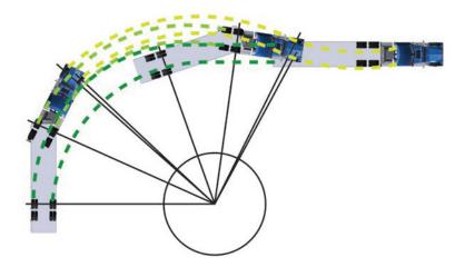
In backing a tractor with a semi trailer, the front wheels of the tractor must be turned in a direction opposite to that in which it is desired to move the rear of the trailer.
